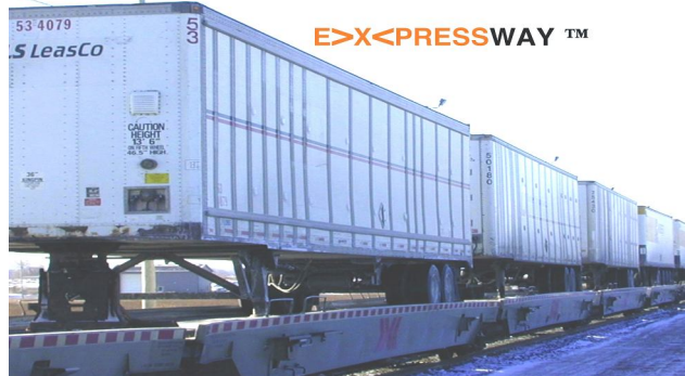
Canadian Pacific E>x<pressway service for trailers
