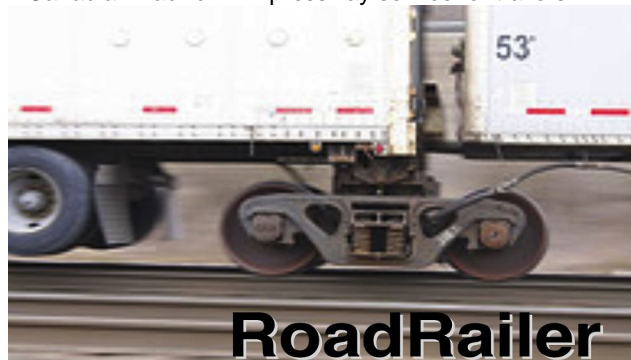
RoadRailer involves putting railroad wheels under trailers
